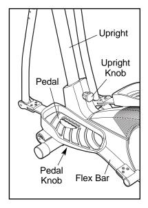
counterclockwise a few turns to loosen it. Next, pull the knob, raise or lower the upright to the desired height, and then release the knob. Move the upright up and down slightly until the pin on the knob snaps into one of the four adjustment holes in the upright. Make sure that the upright is not resting on top of the pin. Then, turn the knob clockwise until it is tight.
